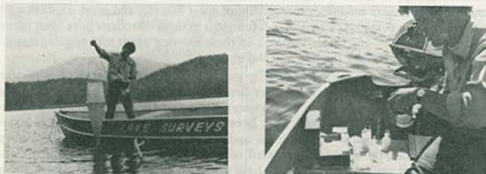
Lake survey crews each summer collect minute forms of aquatic animal and plant life with fine-meshed plankton net (left). Contents are measured for indication of quantity and quality of fish food in each lake. Dissolved oxygen, acidity, alkalinity, and dissolved solids are also measured (right) to determine suitability of each lake for fish life.
